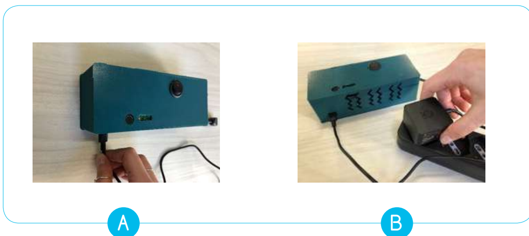
Figure 18: A) power supply hole location, B) connection of the Bedroom Box Case plug in the closest socket.
