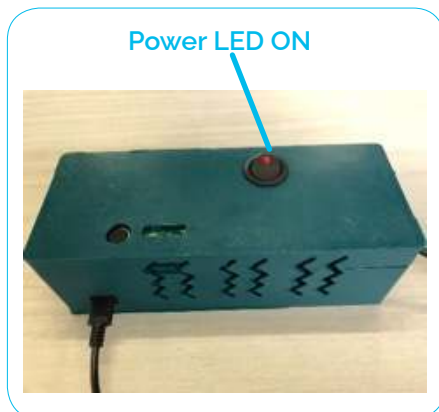
Figure 19: Power LED ON indicates the correct activation of the Bedroom Box Case
