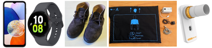
Fig. 1. TOLIFE monitoring devices, from the left to right: SmartPhone (Samsung Galaxy A14), SmartWatch (Samsung Galaxy Wear 5), SmartShoes, Smart Mattress cover, Environmental unit and Spirometer (Smart One OXI)
